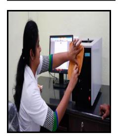
This enables in identification of color of the liquid based on which dyeing composition, effluent analysis and shade sorting can be done.
