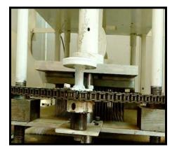
The process of compacting short staple fibers using needles and punching the created lap for further non-woven application can be done using this instrument.
