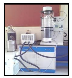
Nano spray is used for giving finish to the fabric after converting the source solution into nano particles
